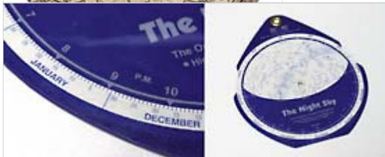
Left: To set the planisphere for a particular date and time, turn the moveable disk until the two (9 p.m. on January 1st in this example) line up with one another. Right: Set thus, the planisphere quickly tells you what constellations are above the horizon. Sky & Telescope / Craig Michael Utter
